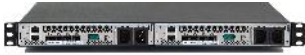
Figure 1. Loxoll Versatility. HA appliance uses hardware-based mirroring to provide redundant data path access to mirrored storage volumes. In the unlikely event of component failure, HA instantly fails over to the working data path and storage. The result: and applications continue running without interruption or manual intervention.
